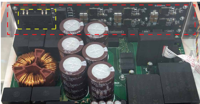
The part of the PCB marked with red is the section that includes SanRex power semiconductors. The product with yellow-marking shows the placement of our DF60NB160.
